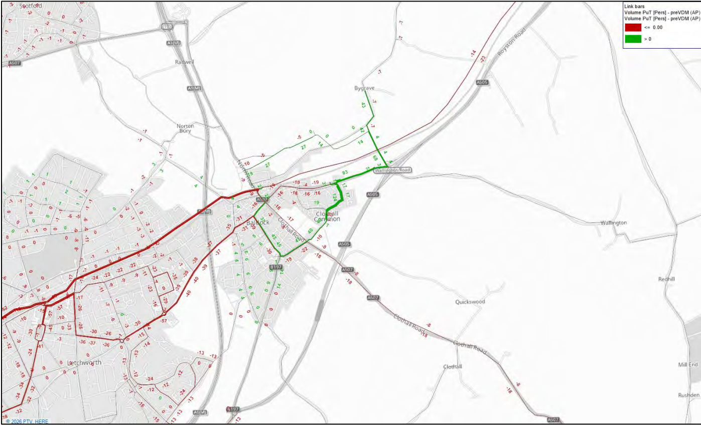
Figure 98: Public Transport Flow Difference Scenario S3-1 (2043 NTEM with development option 1) Post-VDM minus Pre-VDM AM Peak
