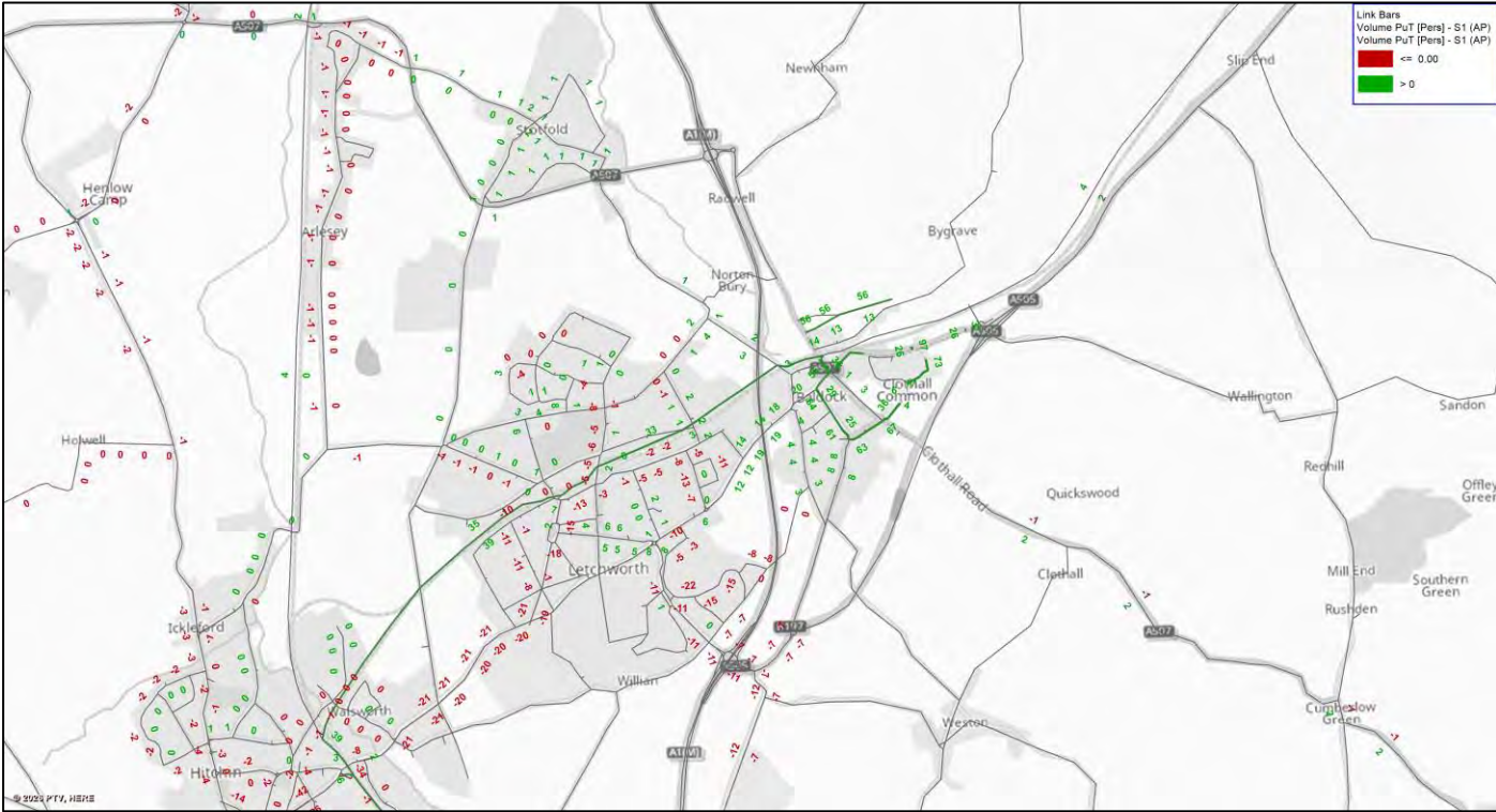
Figure 78: Passenger Flow Difference Scenario S2 (2029 NTEM with interim development) minus Scenario S1 (2029 Do Minimum) PM Peak
