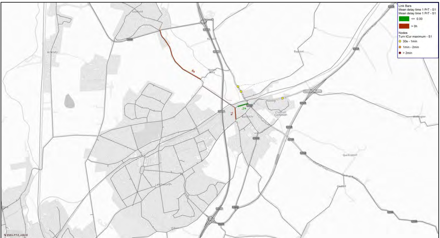
Figure 37: Link and Node Delay Difference Scenario S2 (2029 NTEM with interim development) minus Scenario S1 (2029 Do Minimum) AM Peak
