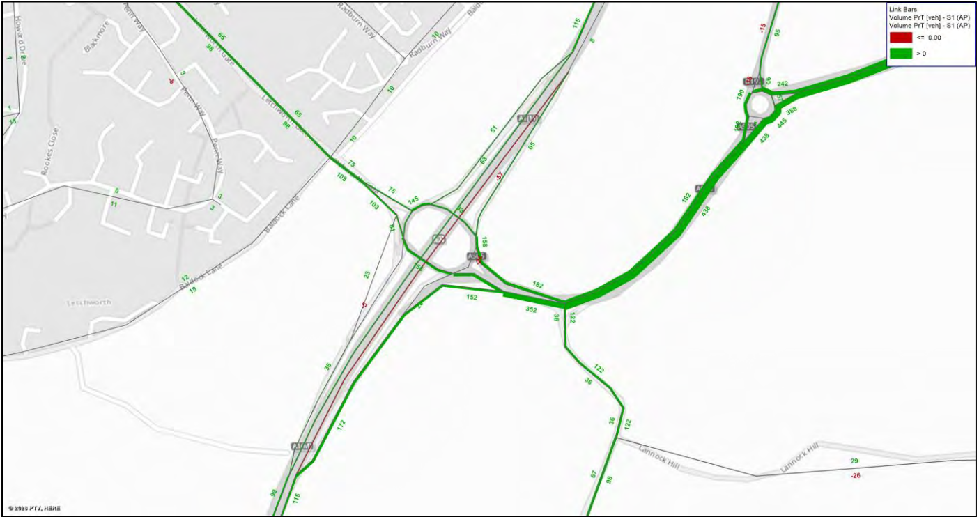
Figure 69: A1(M) Junction 9 Flow Difference Scenario S3-2 (2043 NTEM with development option 2) minus Scenario S3DM (2043 NTEM Do Minimum) AM Peak
