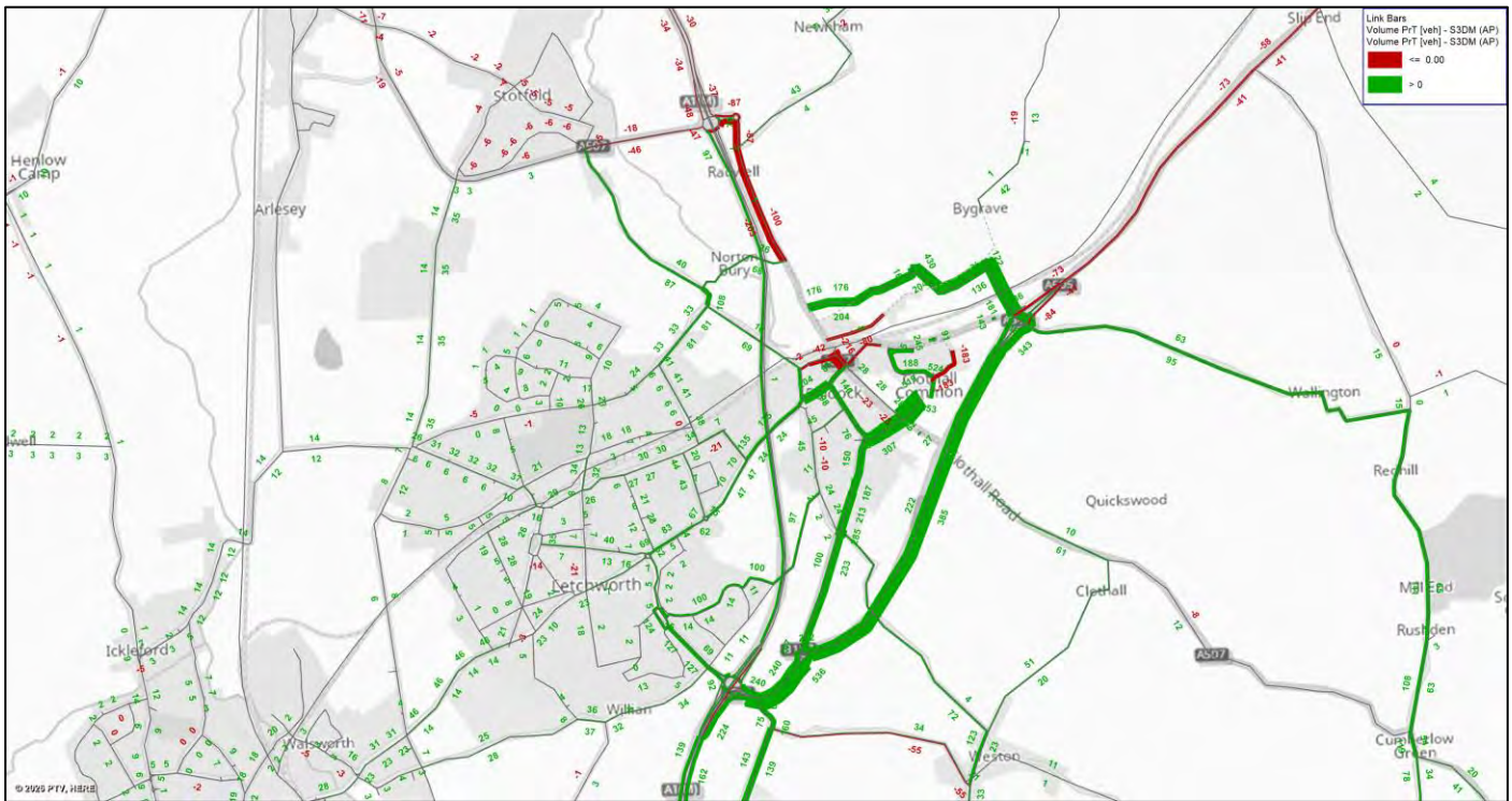
Figure 31: Flow Difference Scenario S3-1 (2043 NTEM with development option 1) minus Scenario S3DM (2043 NTEM Do Minimum) AM Peak
