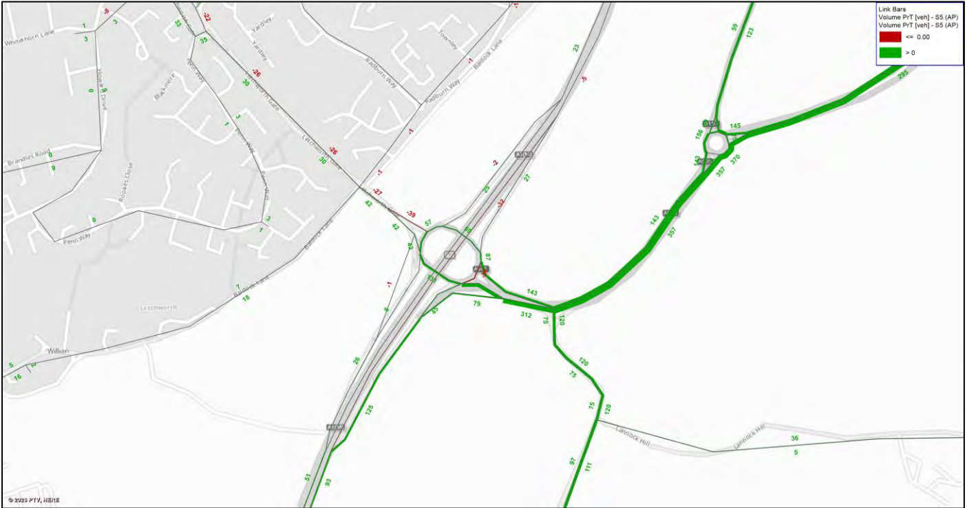
Figure 75: A1(M) Junction 9 Flow Difference Scenario S6-1 (2043 LP with development option 1) minus Scenario 5 (2043 LP Do Minimum) PM Peak
