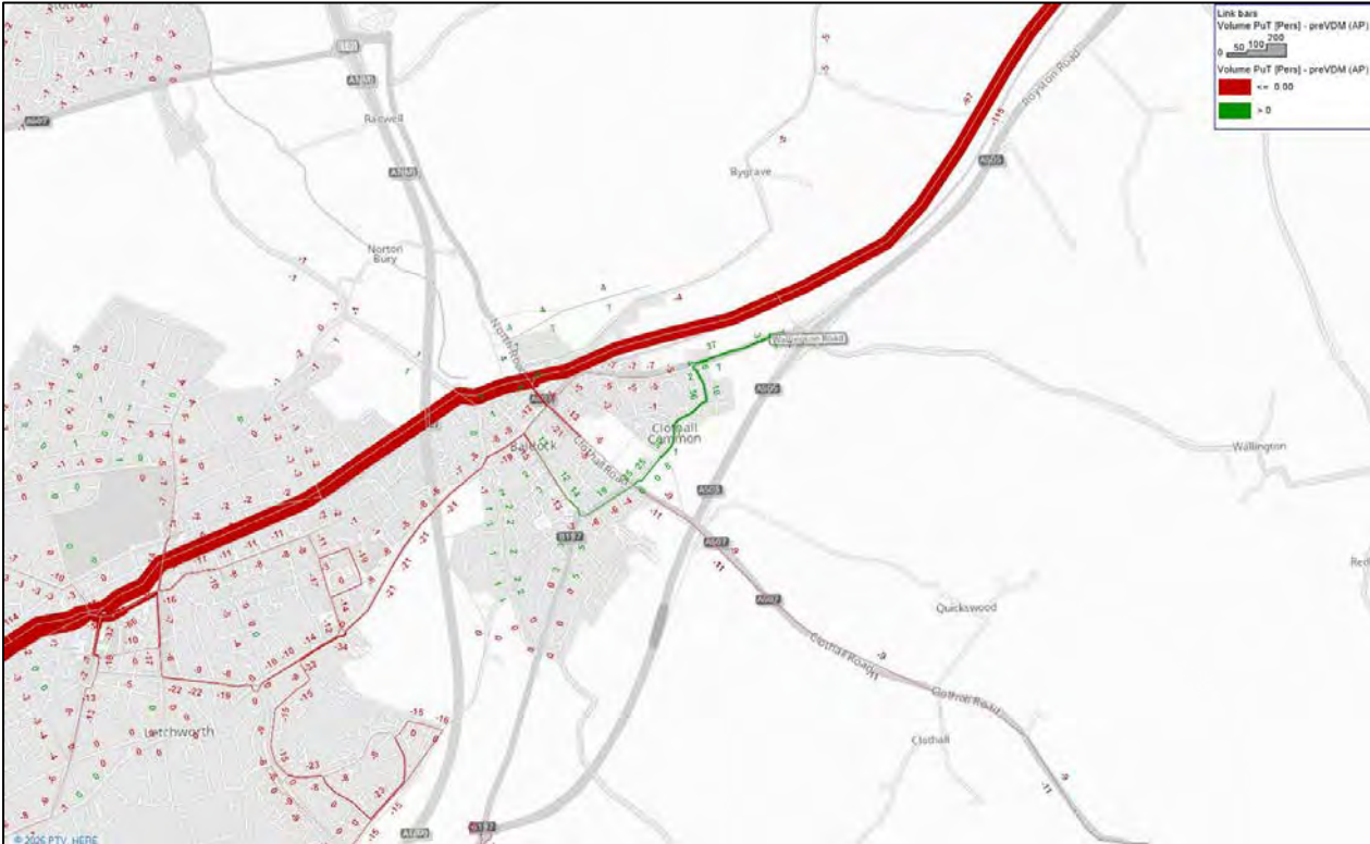
Figure 94: Public Transport Flow Difference Scenario S2 (2029 NTEM with interim development) Post-VDM minus Pre-VDM AM Peak
