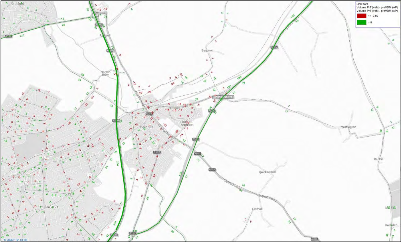
Figure 97: Highway Flow Difference Scenario S3-1 (2043 NTEM with development option 1) Post-VDM minus Pre-VDM AM Peak
