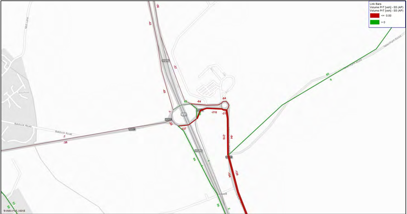
Figure 74: A1(M) Junction 10 Flow Difference Scenario S6-1 (2043 LP with development option 1) minus Scenario S5 (2043 LP Do Minimum) AM Peak
