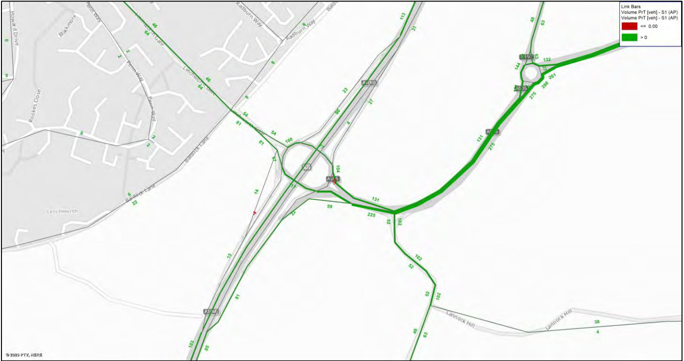
Figure 71: A1(M) Junction 9 Flow Difference Scenario S3-2 (2043 NTEM with development option 2) minus Scenario S3DM (2043 NTEM Do Minimum) PM Peak
